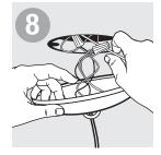
Continue to support fixture. Make sure all connected wires are carefully placed inside box and canopy.
