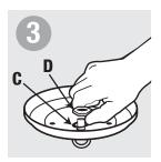
Secure from inside of canopy with washer (C) followed by nut (D). Tighten.
