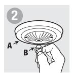
Insert loop (B) into hole from outside of canopy (A).
