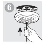
Pass wires from fixture up through hole in loop to inside of canopy.
