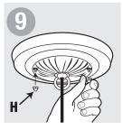
Cover with canopy and secure with cap nuts (H).
