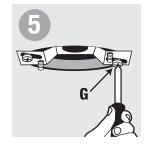
With raised side of crossbar towards ceiling, mount crossbar by inserting 1/2" mounting screws (G) through slotted holes. Tighten until crossbar is flush with ceiling.
