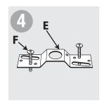
On raised side of offset crossbar (E) thread 1" mounting screws (F) down through each hole that lines up with canopy.
